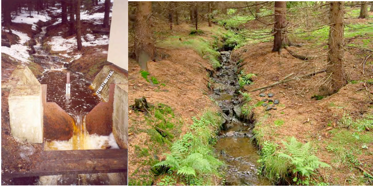
Figure 3. Pluhuv Fig. 3a. V-notch weir during spring snowmelt event. Fig. 3b. Stream channel during summer baseflow conditions
