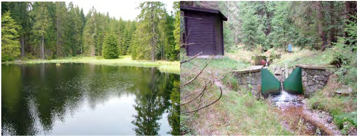
Figure 2. Lysina catchment underlain by granite. Fig 2a. A pond immediately below the Lysina catchment. Fig. 2b. V-notch weirs on the main stream during baseflow conditions.
